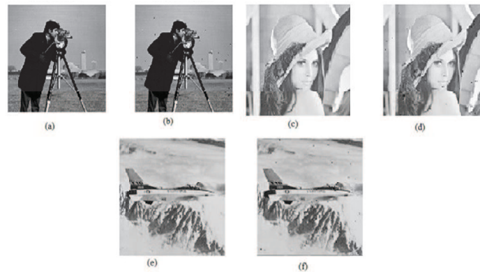
Figure 6. (a) Original Image of cameraman (b) Reconstructed image with CSNR 20 dB with reduced Approximation noise. (c) Original Image of lena (d) Reconstructed image with CSNR 20 dB with reduced Approximation noise. (e) Original Image of airplane. (f) Reconstructed image with CSNR 20 dB with reduced Approximation noise
