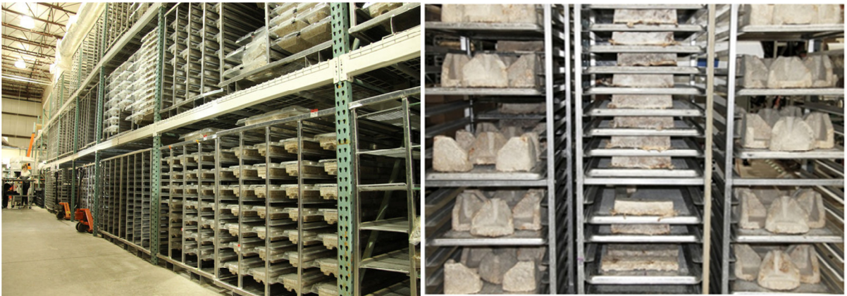
Fig. 2. Production facility for mushroom based foam
